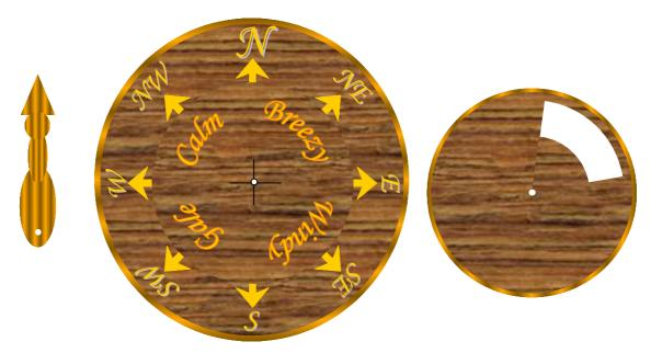
Cut out the above Binnacle parts, including the white space on the smaller dial and glue each of them to card. Then mount the smaller dial on the larger, and finally the arrow on top, all held together with a bent-over drawing pin through the centre (white) spot. The smaller dial is then used to track wind speed (Calm, Breezy, Windy, Gale) whilst the large arrow is used to track wind direction.
